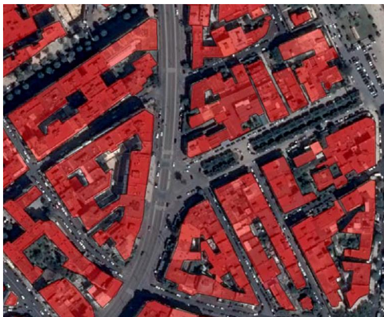
EO derived urban blocks manual mapping over Rabat/Sale, Morocco Source: Pléiades © CNES 2019, distribution Airbus DS
