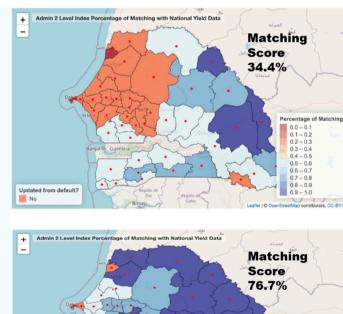
**Lower image:** an NGDI design set-up consisting of two measurement windows in the season (early and late) with two indicators combined – satellite-based rainfall and soil moisture, and a resulting much higher matching score (agreement of satellite data with reported drought years), going from 34.4% to 76.7.
